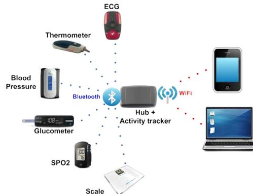
Fig. 3. Wireless gateway for RPM.
